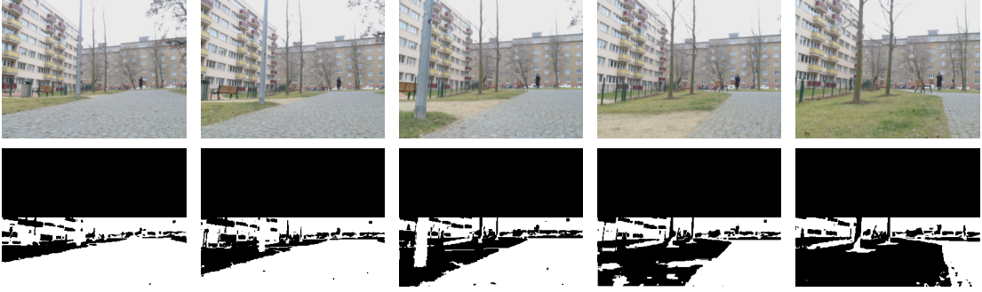
Figure 22 The results of the GMM based road detection in experiments with robot. Figure contains 5 evenly distributed images from DS3 and corresponding found paths.
