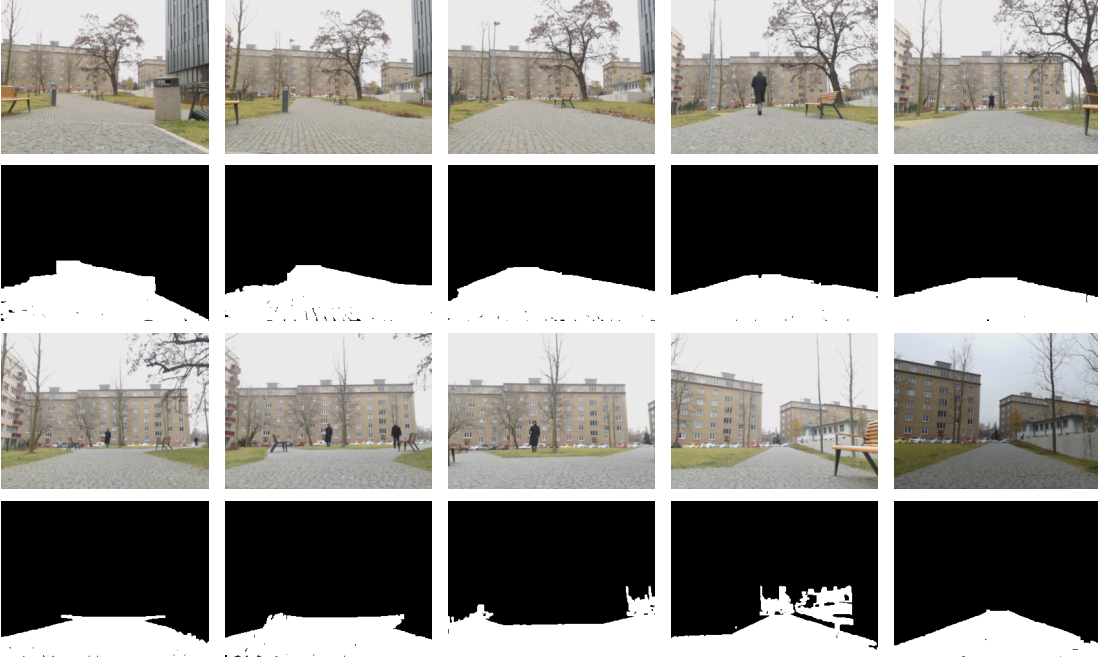
Figure 21 The results of the combined method of road detection in experiments with robot. Figure contains 10 evenly distributed images from DS3 and corresponding found paths.
