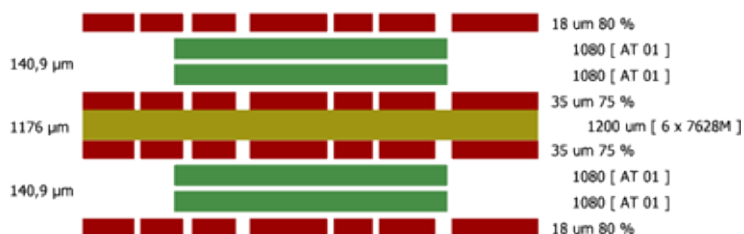
Figure 30 Cross section of a four layer pcb made by Pragoboard [26].
