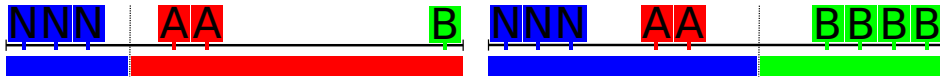
Figure 7.2: Example how SMOTE can expand the decision region of negative class during node splitting when SMOTE is applied on positive class. The figure on the left shows how decision tree would split three classes based on entropy. If the child nodes were leaves the left leaf would classify objects as negative ( N ) and the right leaf would classify objects as positive class A . In the right figure, 3 synthetic samples were created by SMOTE to positive class B . This forces the decision boundary to move and as a result the region which classifies objects as negative is larger than in the left figure.
