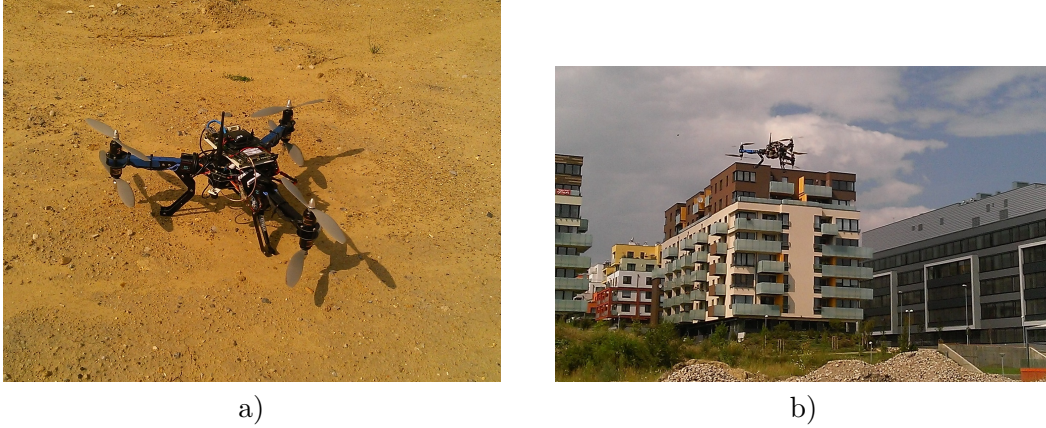
Figure 3.2. Y6 hexacopter used to acquire data.
