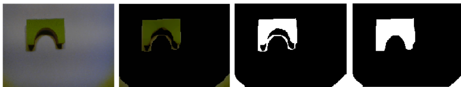
Figure 6.10: Image processing – original image, removal of the background, converting to BW image and filling the holes for the images acquired through iCub simulator and physical iCub.
