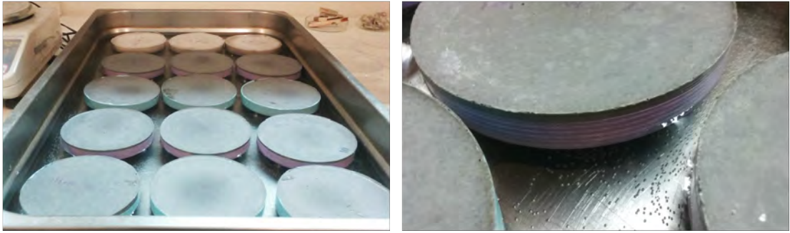
Fig. 17: Arrangement of the surface water absorption test
