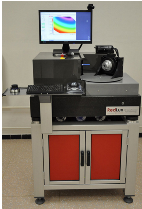
Figure 3.1: Optical 3D CMM by RedLux Ltd. ( http://goo.gl/veqx5V )
