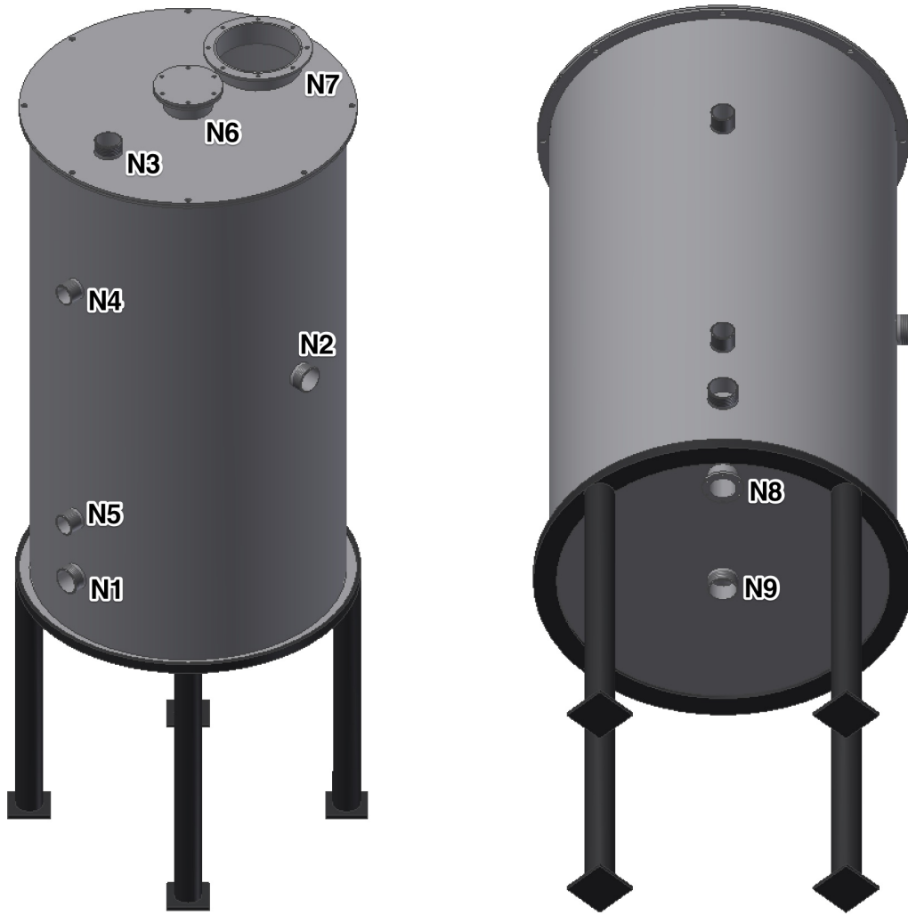
Fig. 26 Retention vessel 3D model, N1 – mixture inlet, N2 – mixture outlet, N3 – fresh medium inlet, N4 – heat exchanger inlet, N5 – heat exchanger outlet, N6 – stirrer attachment, N7 – gas outlet, N8 – gas inlet, N9 – processed medium outlet
