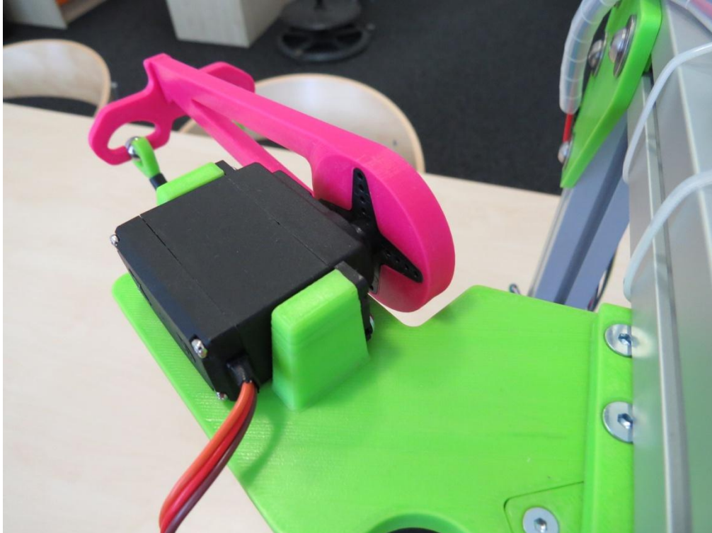
Obr. 27: Detail serva MG996R
