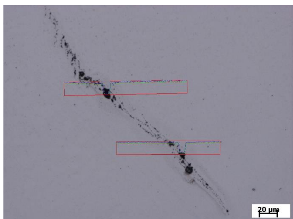
Obr. 73 - Mar M246 + X22CrMoV12 - trhlina
