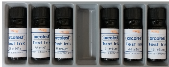
Figure 2.1: Arcotest test inks for measuring of surface energy
