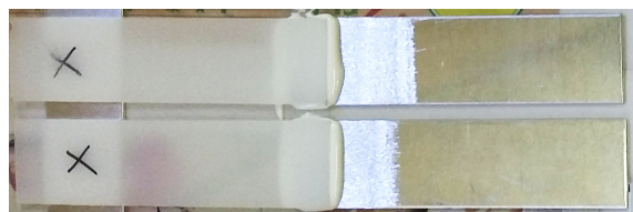
Figure 2.3: Samples adjustment for curing (on the left side the aluminium underlay can be seen)
