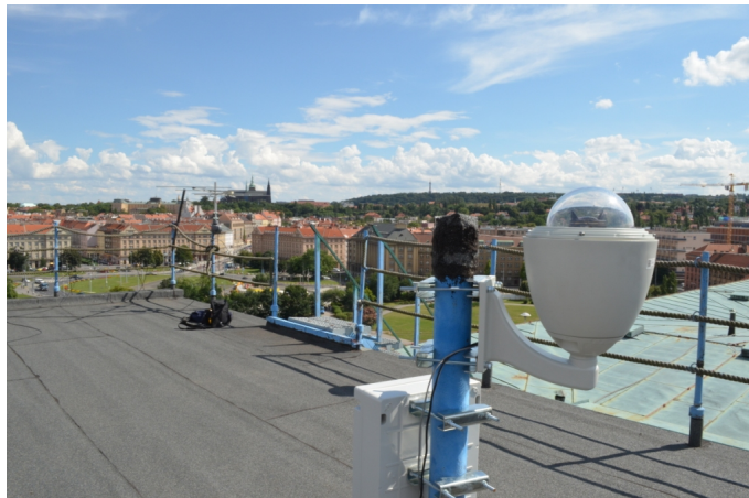
Figure 14: Project WILLIAM - Wide-field all-sky image analyzing monitoring system - run by Multimedia Technology Group of Czech Technical University.
