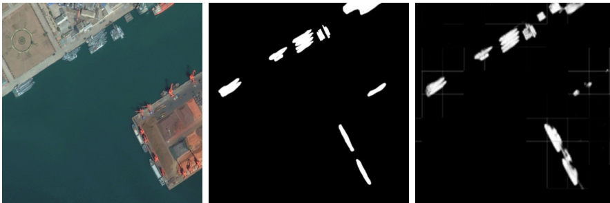
(b) : Image size: 1k x 1k pixels, resolution: 0.5m, provider: Digital Globe. The largest ships are about 170 pixels long. We can see that the network does very well for ships this size and resolution.
