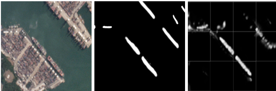
(c) : Image size: 500 x 500 pixels, resolution: 3-5m, provider: Planet Labs. The algorithm attempts to generalize to images at this resolution even though such images are not in the training set.
