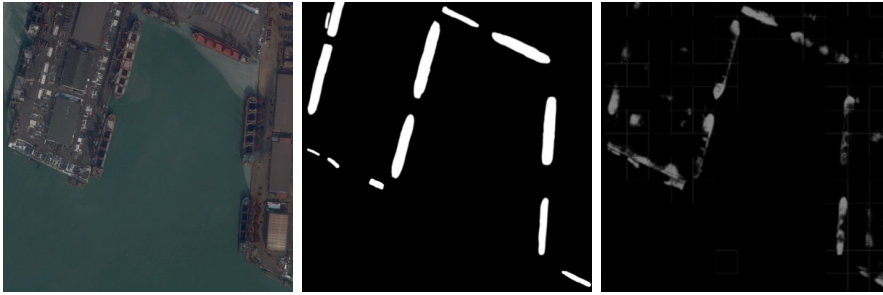
(a) : Image size: 2k x 2k pixels, provider: Digital Globe, resolution: 0.5m. Big ships are up to 500 pixels long which is too big for the 255 \times 255 context window. We can see that the network detects the characteristic bow and stern of the ships but is unable to discern the bay most of the times.
