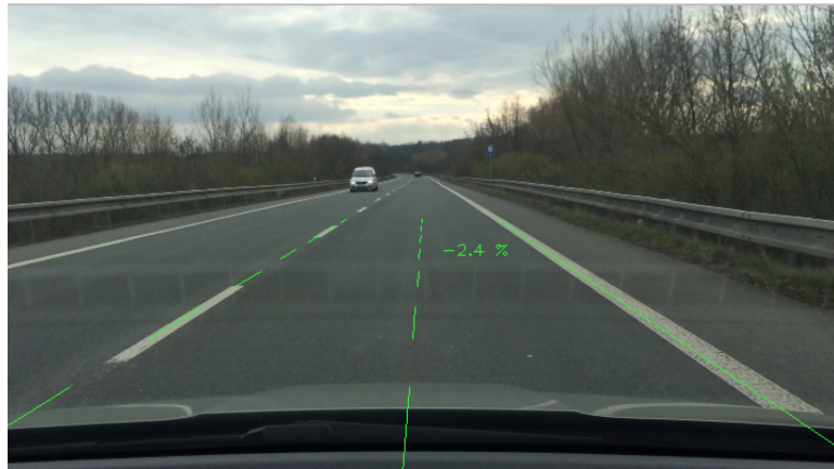
Figure 3.1: Example of successfully detected lane in the country road
