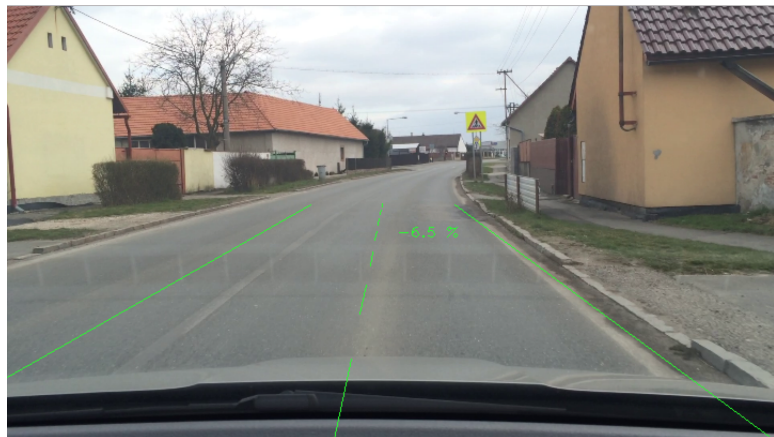
Figure 3.5: Example of erroneous detection caused by faded left marking
