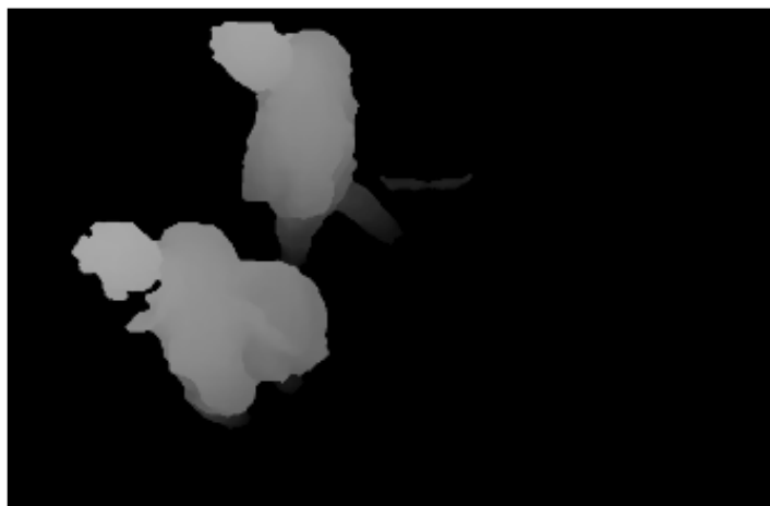
Figure 3.2: Example of depth map with two humans. Note one of them is pulling a shopping basket.
