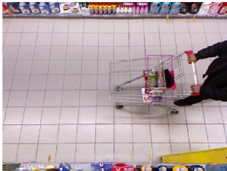
Figure C.4: Example of too small bounding rectangle which the CNN recognizes as containing a cart.
