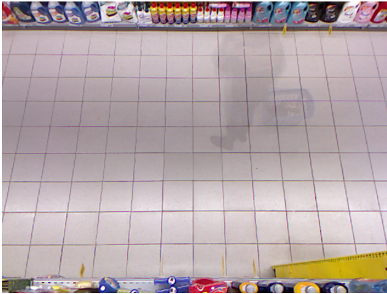
Figure 3.4: Example of background image with a ghost caused by a human standing for a long time at one place.
