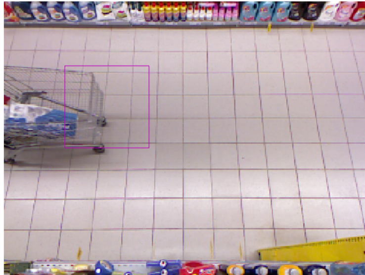
Figure C.3: Example of a partially matching bounding rectangle which the CNN recognizes as containing a cart.
