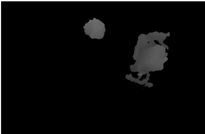
Figure C.6: A problematic image for human detection, depth counterpart to C.5. Note that there is large cluster representing a cart and that the right human is not visible in the depth map at all.
