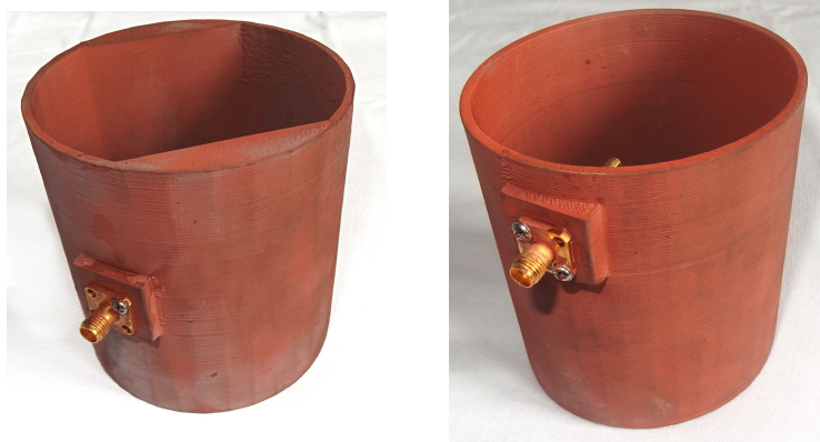
Figure 87: Circular and elliptical polarizers with copper coating.
