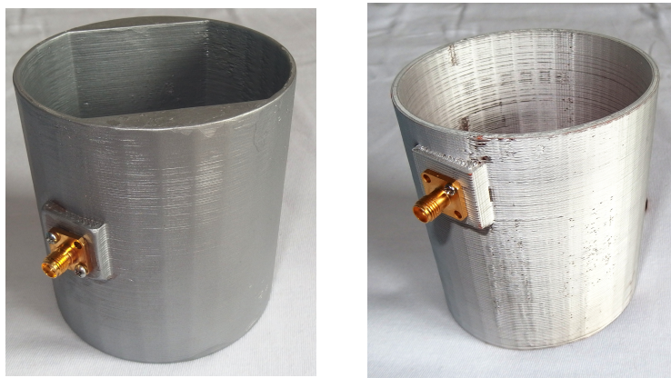
Figure 88: Circular polarizer with vacuum metallizing and elliptical polarizers with aluminium spray.
