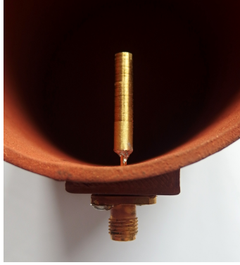
Figure 86: The view of the attached connector with probe.
