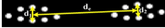
Figure 3.7 Eye openness degree is computed as a ratio between height of the eyes and a distance between eyes in [37].
