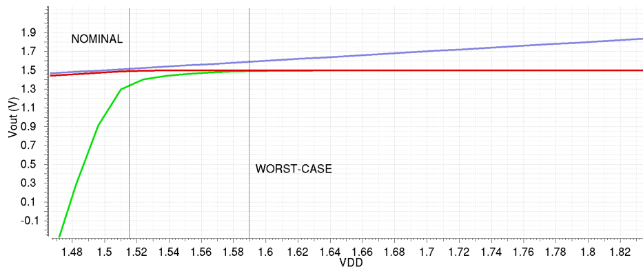
Figure 5.7: Input voltage sweep - dropout and regulation region
