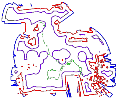
(a) : The polygonal map (obstacles - red, frontier - blue, expanded - violett / grey) with a path of the robot (green).
