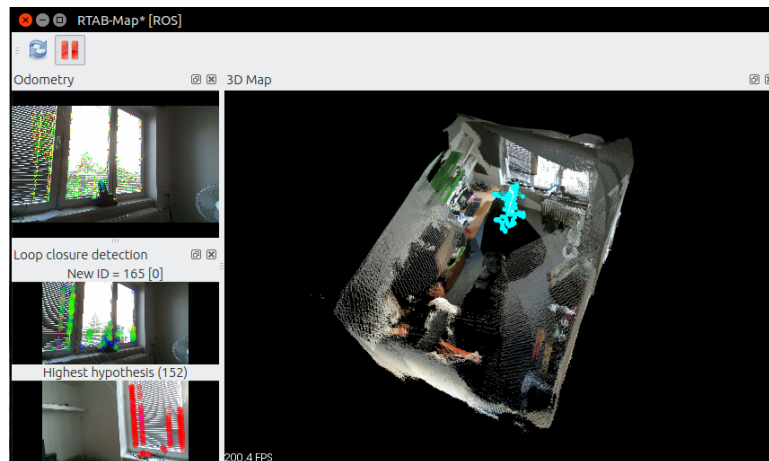
Figure 3.13: RTAB-Map used with a hand-held Kinect2 sensor in a small room.
