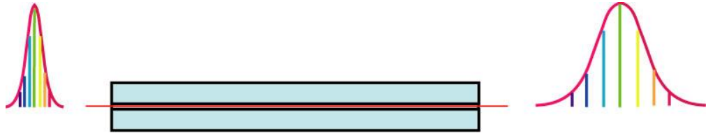
Fig. 2.1.1: Effect of Chromatic dispersion on the wavelength components of the launched pulse [11].
