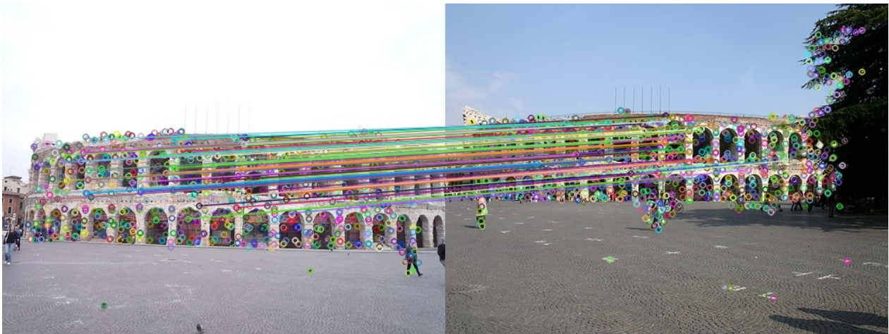
Figure 5: Example of identified matches using AKAZE detector and knn matcher
