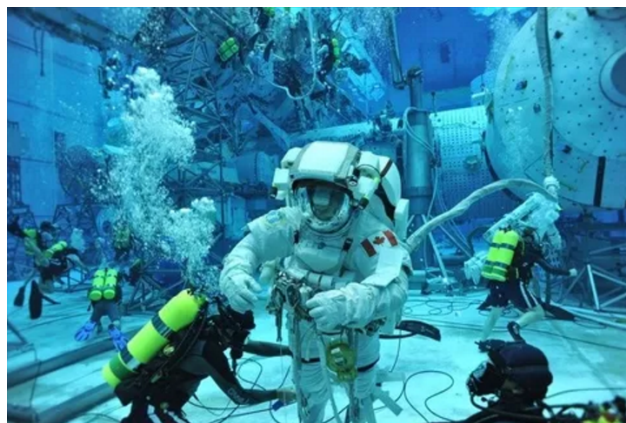
Figure 4: Neutral Buoyancy Laboratory operated by NASA in Houston features a model of ISS for astronaut training. Photo: NASA .
