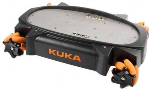
Figure 11: Youbot from Kuka. It provides unconstrained planar movement with the use of mecanum wheels.
