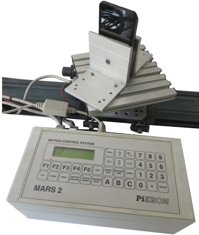
Figure 2.8: Measuring setup - MARS 2, rotation table with
