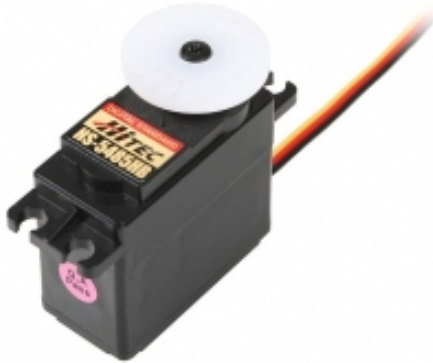
Figure 1.9: Powerful Hitec servo that will actuate the camera. 4
