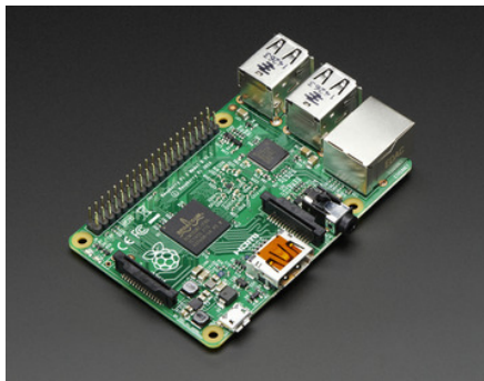
Figure 1.12: Small, inexpensive Linux-based computer Raspberry Pi 2 Model B. 5
