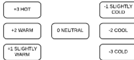
Figure D.6 : Indoor environment thermal states according ANSI/ASHRAE Standard 55-2013, for evaluating PPD by elections, source: Lucidchart design
