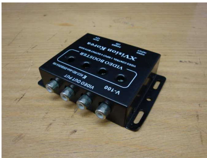
Obr. 3 – Video rozdělovač 1 to 4 Car DVD LCD TV Video Monitor Amplifier Booster Distribution RCA Splitter.
