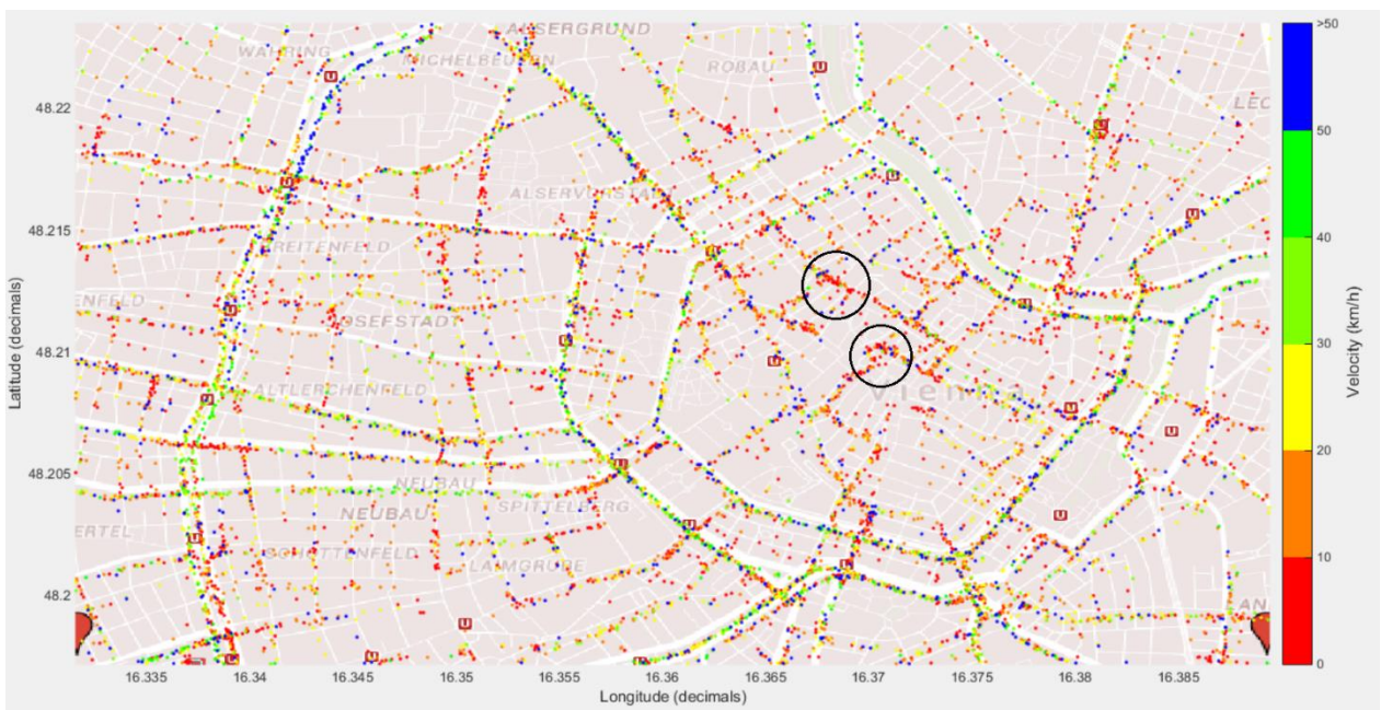
Figure 4.22 Road velocities between 16 and 17 rush hours on Monday with marked congested areas
