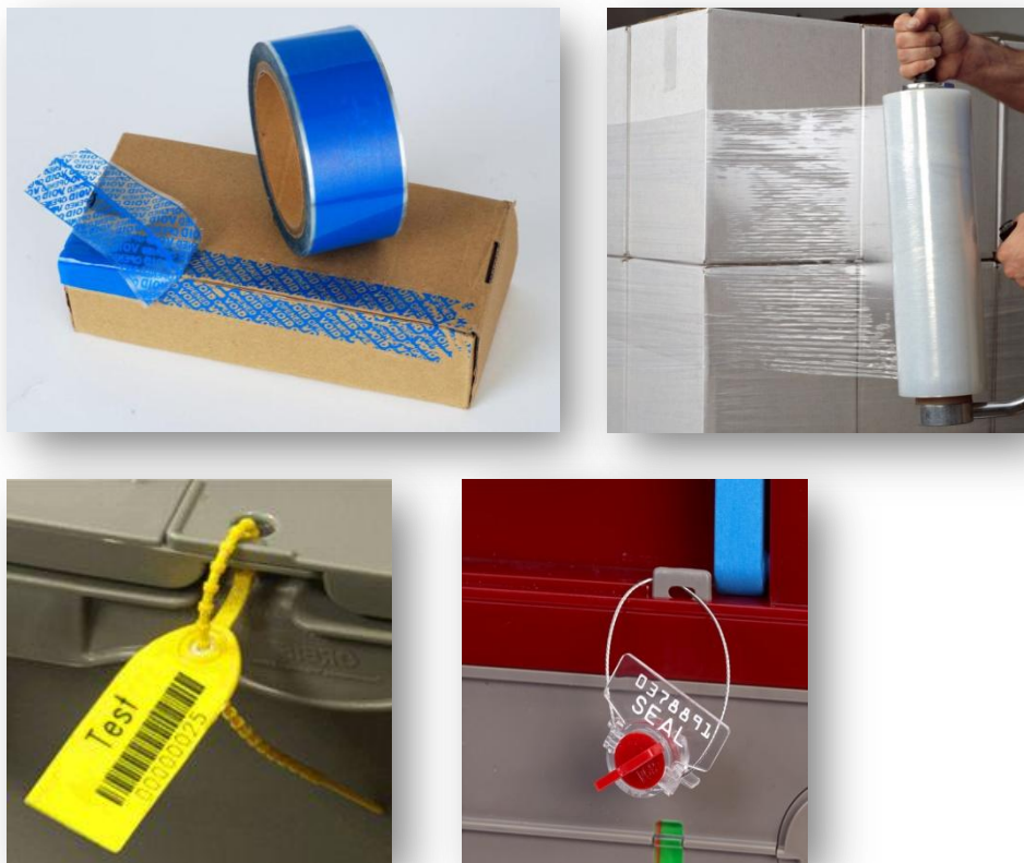
Figure 8: Transport units protection – sealing tape, stretch wrap, pull tight seal, wire seal [Source: interplas.com , diebolddirect.com , fricknet.com ]
