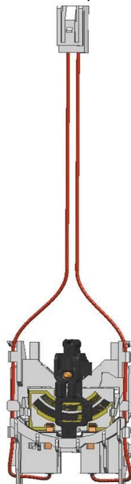
Fig. 2.2 CAD model of FLS assembly (without floater arm).
