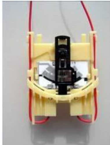
Fig. 1.2 Fuel level sensor without floater arm.
