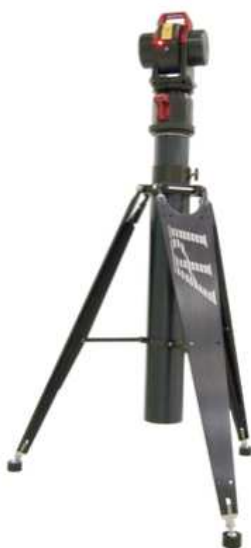
Obr. 3.9 Laser tracker API Omnitrac [10]
