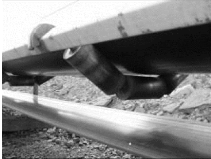
Figure 3.27 Top idlers as flexing units strung by end fixings (Garland idler set) [1]
