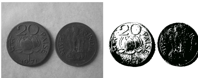
Figure 2.2: Image of coins before (left) and after (right) transformation into binary image [9]. Pixels in original image with intensity lower than 70 are black, others are white.
