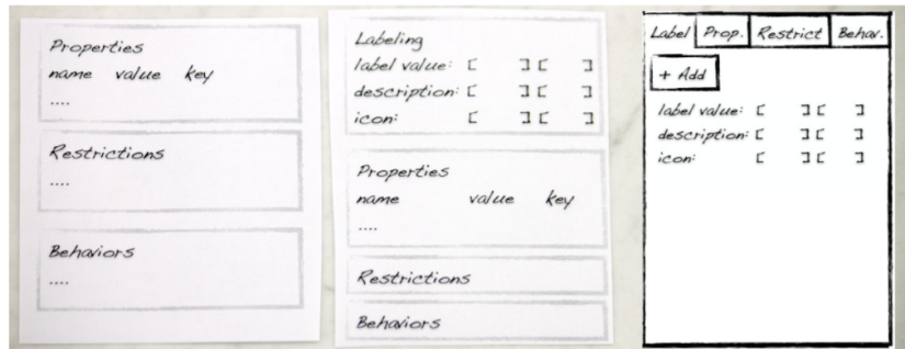
Figure A.4: Evolution of property window of the Low-Fidelity prototype of the UIP Visual Editor , from [42]
