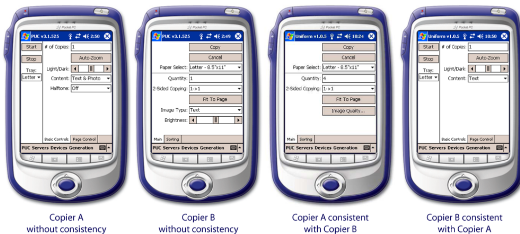
Figure 2.5: User interfaces generated by Uniform tool for a simple and complex copy machine with consistency attribute disabled and enabled (from [72])
