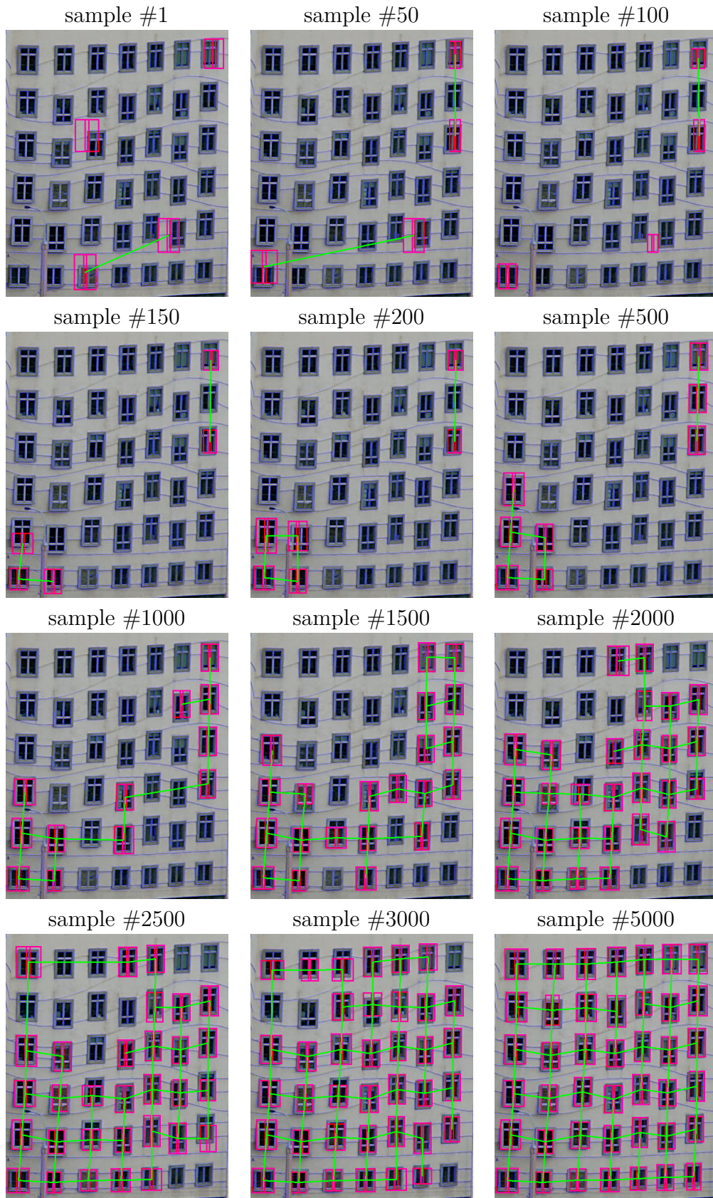
Figure 2.13: Inference progress of the proposed RJMCMC sampler. Detected windows are shown in red, neighborhood edges in green and image edges are emphasized in blue.
