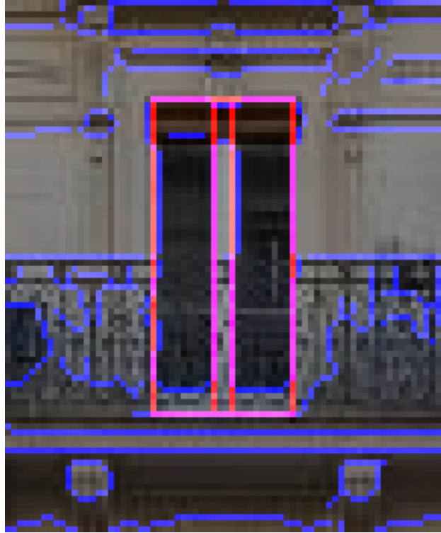
Figure 2.7: The shape template (red) is matched with image edges (blue)
