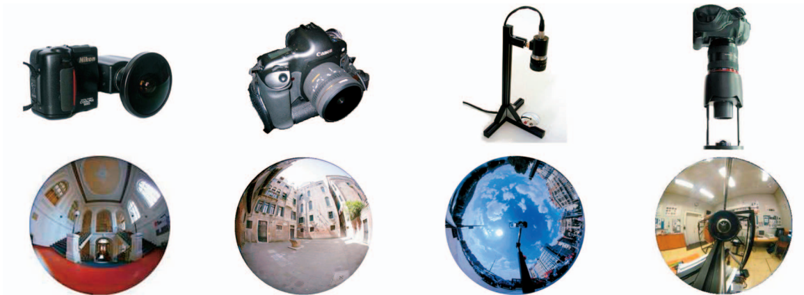
Fig. 1. Omnidirectional cameras and acquired images. From the left: Nikon Coolpix digital camera and Nikon FC-E8 fish-eye lens; Canon EOS-1Ds and Sigma 8mm-f4-EX fish-eye lens; perspective camera and hyperbolic mirror; orthographic camera and parabolic mirror.
