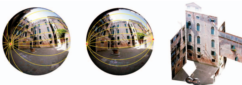
Fig. 2. The 3D metric reconstruction built from two uncalibrated omnidirectional images. Input images with drawn epipolar curves are shown.
