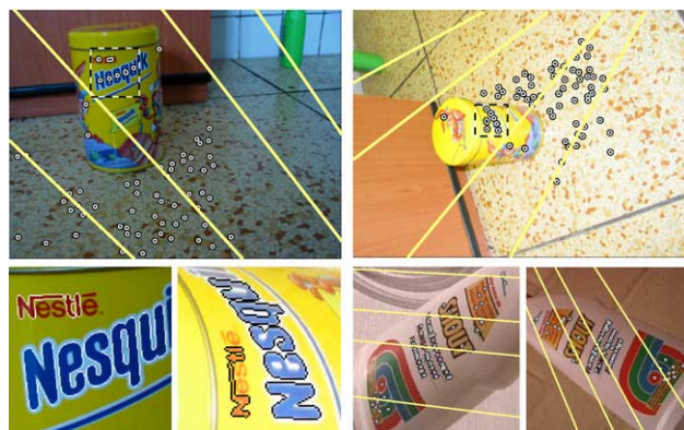
Fig. 5. Cylindrical box. Epipolar geometry (top) and matched regions (bottom left). Fully affine distortion, a non-planar object, textured surface and strong specular reflections are present in the scene. SHOUT (bottom right), a scene with a change of illumination spectral power distribution.
