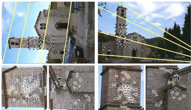
Fig. 2. Valbonne. Estimated epipolar geometry and points associated to the matched regions are shown in the first row. Cutouts in the second row show matched bricks.
