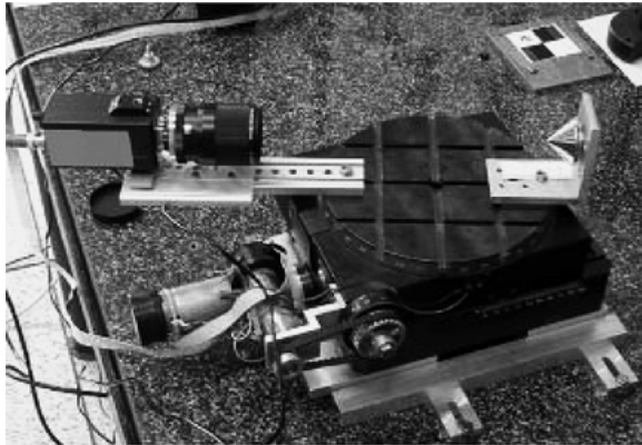
Figure 7. Two sets of rays forming hyperboloidal closures can be realized by rotating catadioptric camera consisting from a telecentric optics and a conical mirror.
