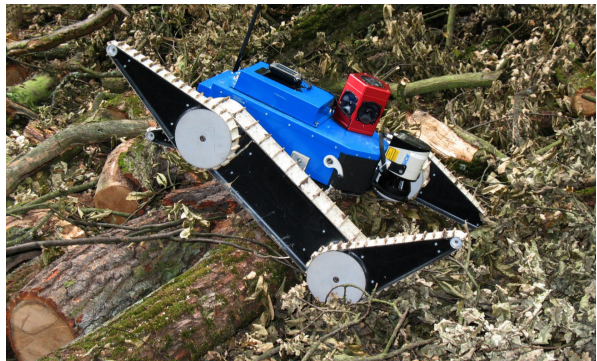
Fig. 1 The skid-steer mobile robot. See Section 3 for details about the sensory set and multi-modal data fusion.
