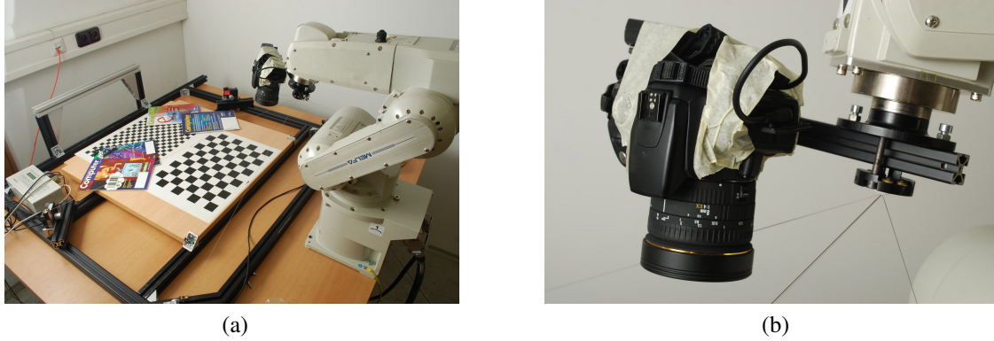
Figure 5.1: Hand-eye calibration robotic setup. (a) A Mitsubishi MELFA-RV 6S serial manipulator equipped with a Canon 350D DSLR camera. (b) Detail of the hand-eye setup.
