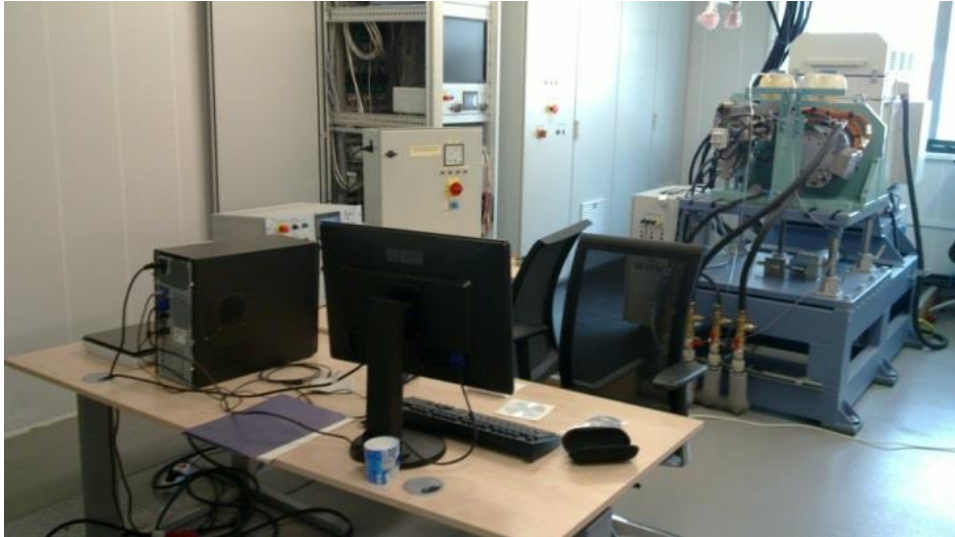
Figure 6-2: Laboratory of EV's and HEV's electric drives measurement – dynamometric test bench is on the right and power supply rack with control PC is on the left.
