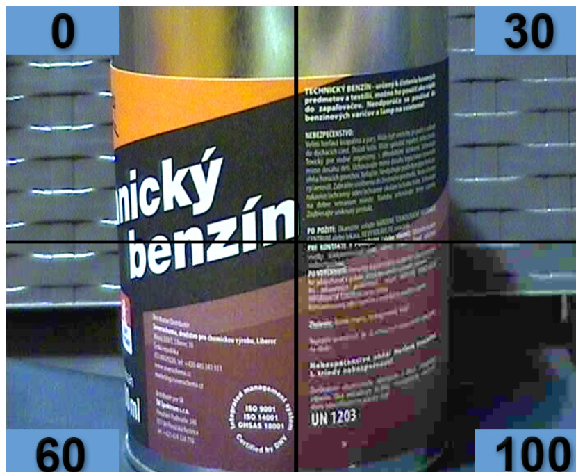
Figure 6.4. Four selected levels of compression show how the compression affects the visual quality of the image. The values up to level 30 are almost indistinguishable. The values between 30 and 60 are still applicable but the reduction in quality is visible. The values greater than 60 should not be used.
