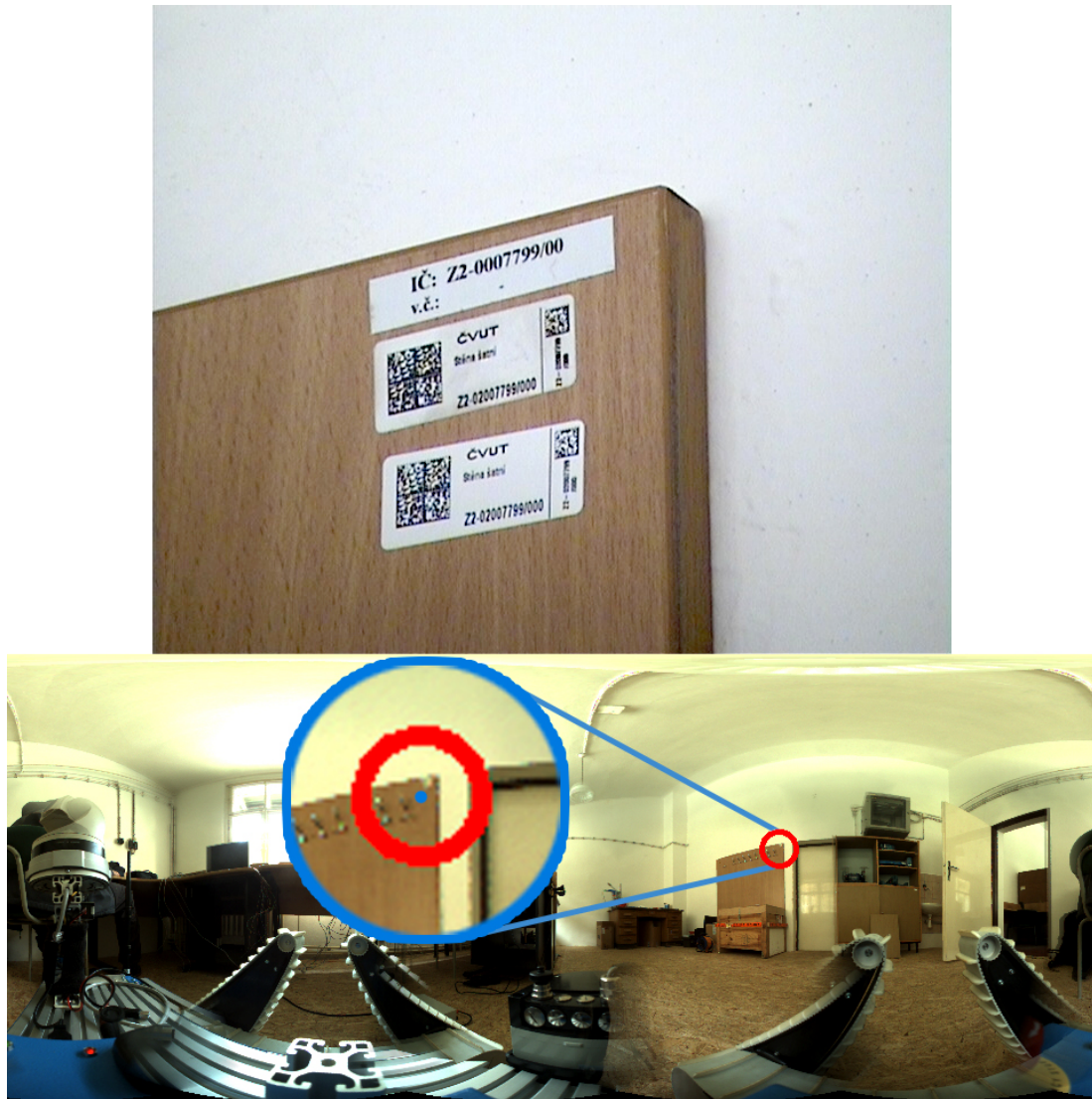
Figure 6.9. An example shows the scene where the point of interest is 3 m far. The enlargement part of the picture shows that the error between the wanted and the real position is approximately 7 pixels. The error is greater for objects near the robot. But the concept of navigation used by mouse_telop is to click on the panoramic image for receiving a widescreen image from PTZ camera. The widescreen image is not as susceptible to the error as an enlarged image. Then it is already possible precisely tuning position by image from Axis camera. Moreover the widescreen image is good for operator orientation.
