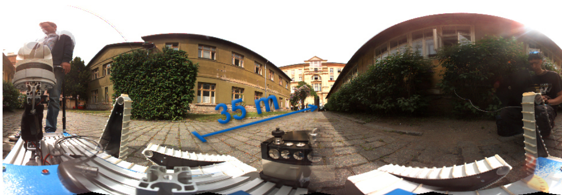
Figure 6.2. Spherical image from Ladybug – operator lacks an optical zoom function. Objects, which are close, may be partially enlarged using a digital zoom. However this is not enough.
