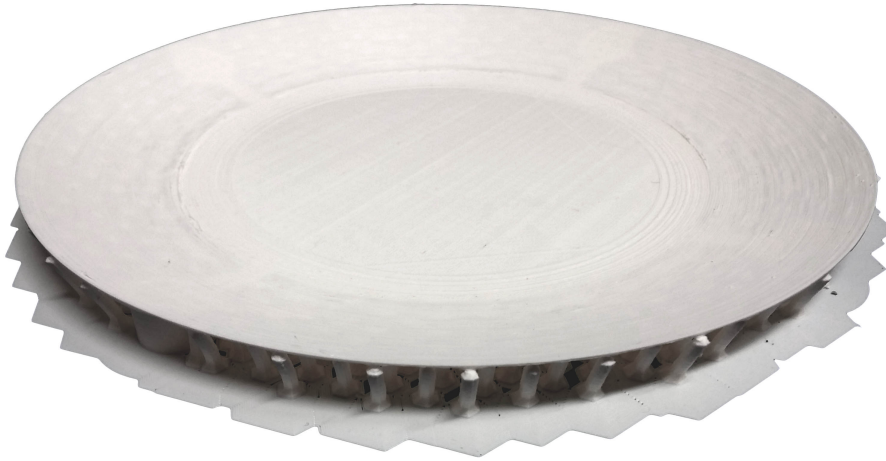
Figure 2.4: Printed surface prior to removal of support structures
