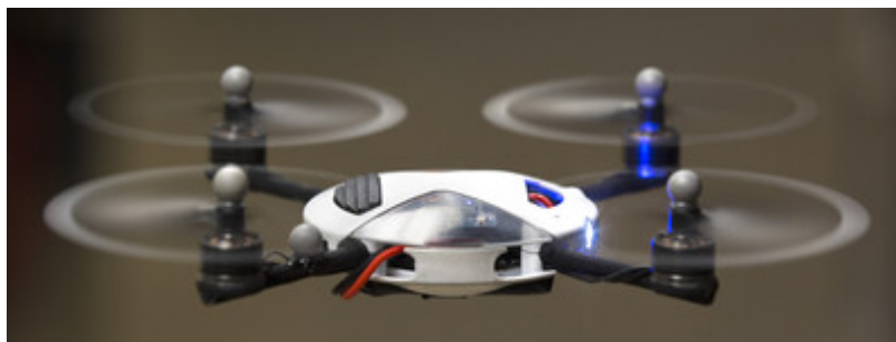
Figure 9: Vicon markers (grey balls at the top of the rotors), Courtesy of [5]
