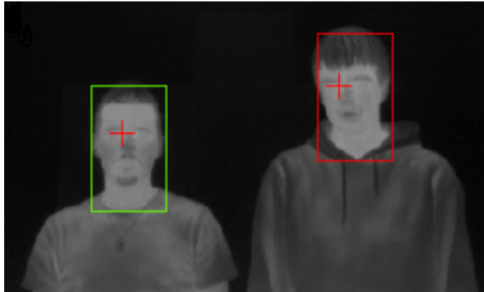
Figure 5.13: An example of detection of the two persons in thermal image. The left one has temperature lower than the limit, the temperature of the right one's is elevated.
