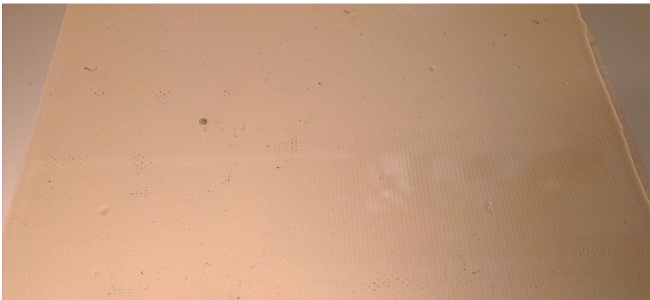
Picture 12-4R: Impurities on RTT's copper board
