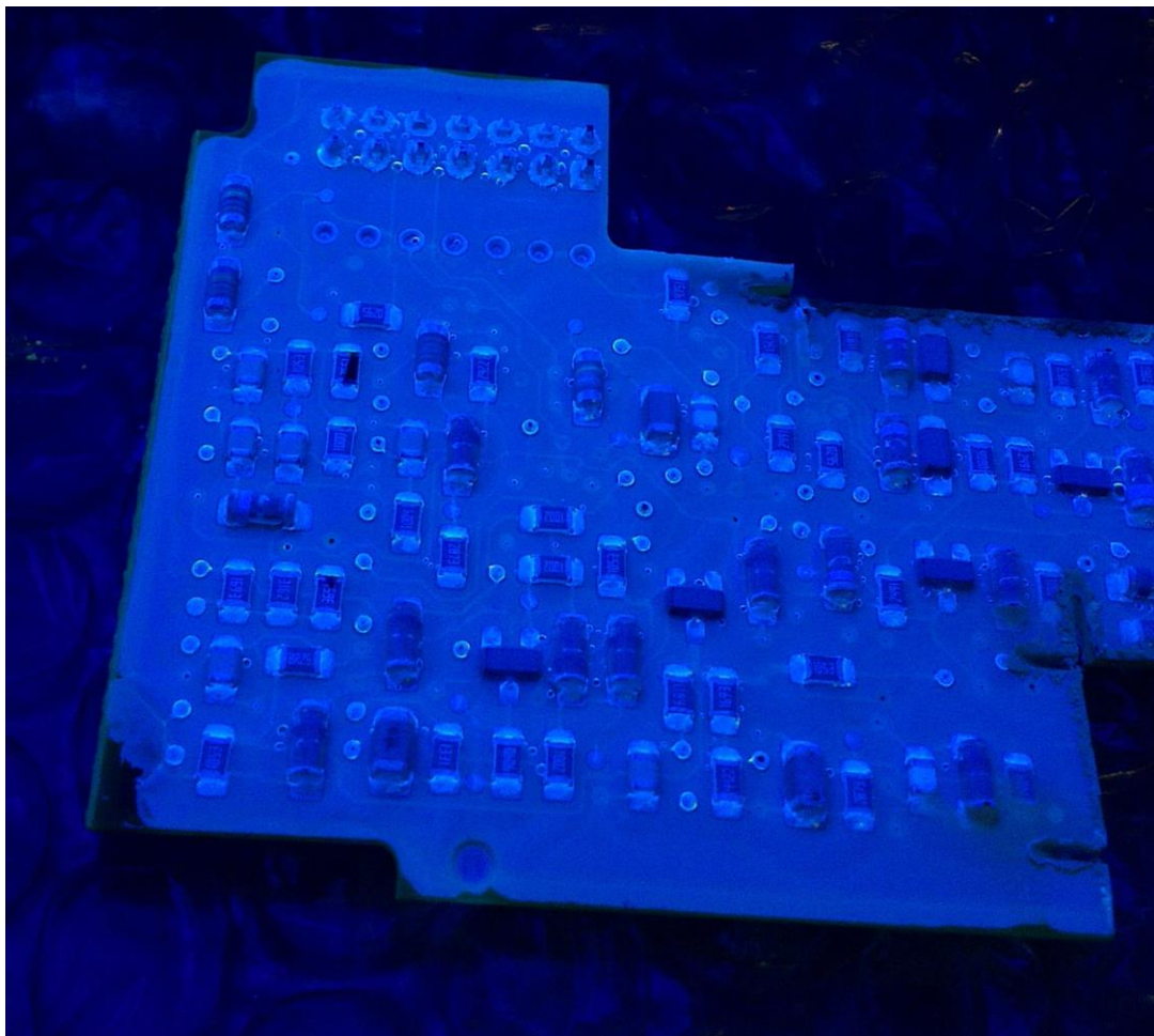
Picture 9-8: Wrinkles – thick, but still not enough for several SMDs (viscosity)
