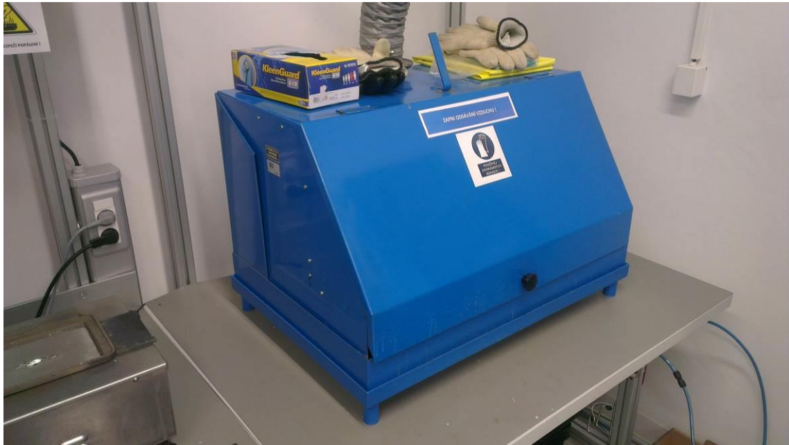
Picture T3: Extraction system necessary during curing time
