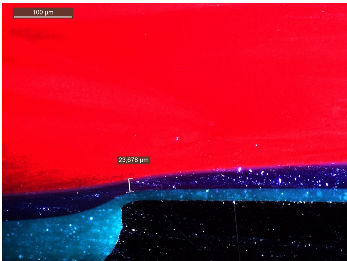
Picture 10-2-2: Layer is relatively equal on the inspected area, critical point
