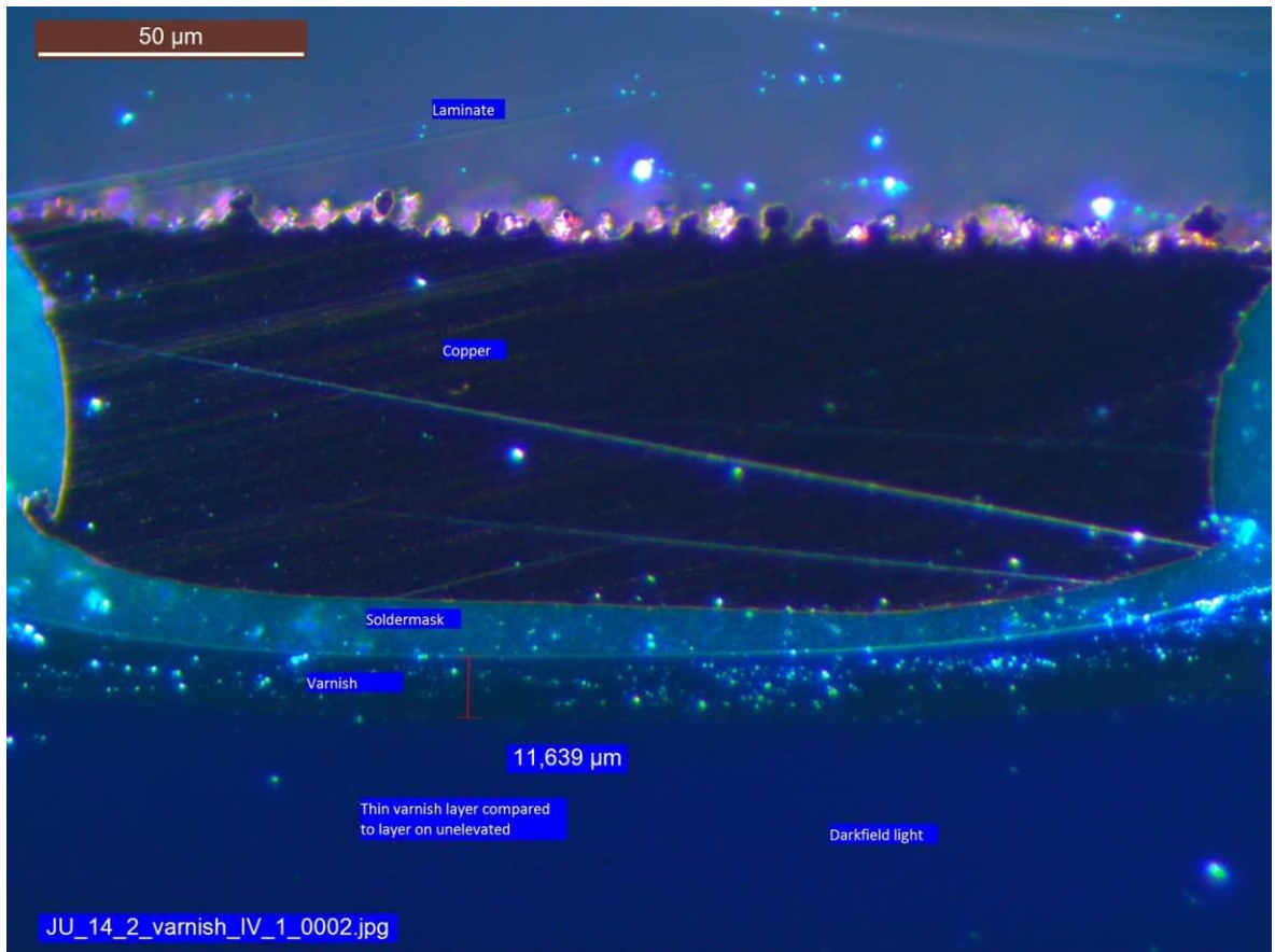
Picture T11: Microsection sample, Darkfield light
