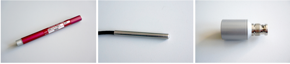
Figure 6.1: The selected and tested tiny "pen" detectors. From the left: the \text{CeBr}_3 detector from Scionix , the CZT#1 detector from Ritec and the CZT#2 detector from Ritec .
