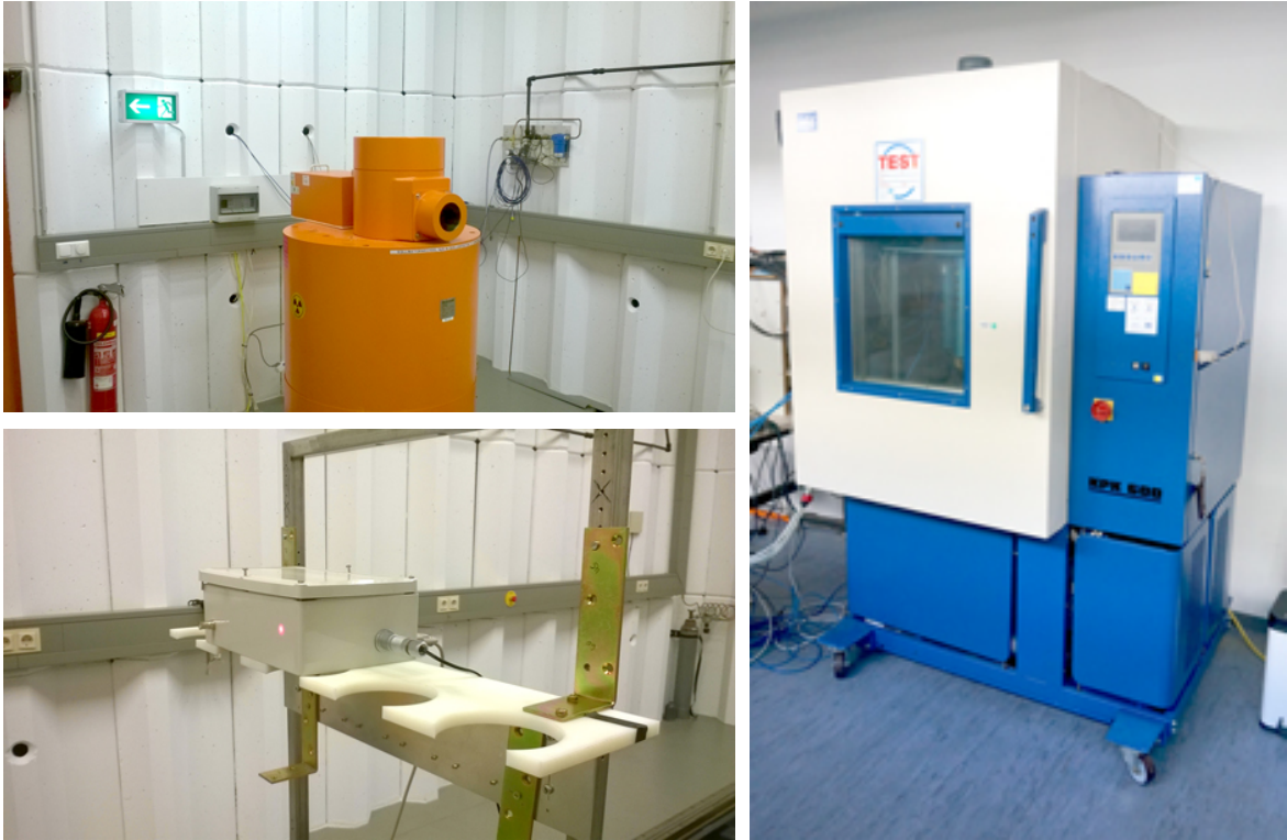
Figure 6.7: The two pictures on the left show the source facility and placement of the detector onto a trolley in the radiation chamber in Munich. The right picture shows the climatic chamber used.
