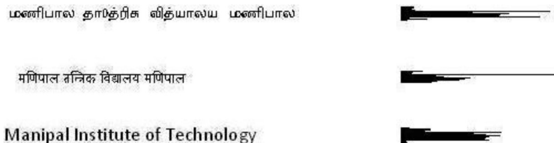
Figure 2.5. Example of horizontal projection profiles for Tamil, Hindi and English lines of text. Notice the distinct peak in Hindi text. Image taken from [21].
