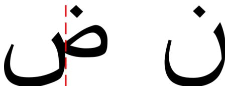
Figure 2.1. Example of an over-segmentation of the letter Dad (left) marked in red dashed line. Although the left part of the segmentation resembles the letter Nun (right), it is missing the diacritical mark, therefore, the segmentation is incorrect and can be removed.
