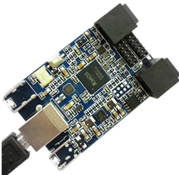
Ilustrace 3.4.1: Modul USBStreamer [24]
