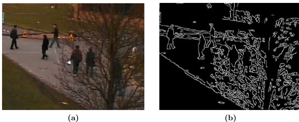
Figure 4: Illustration of edges present in the image background. (a) image from the sequence. (b) corresponding edge image
