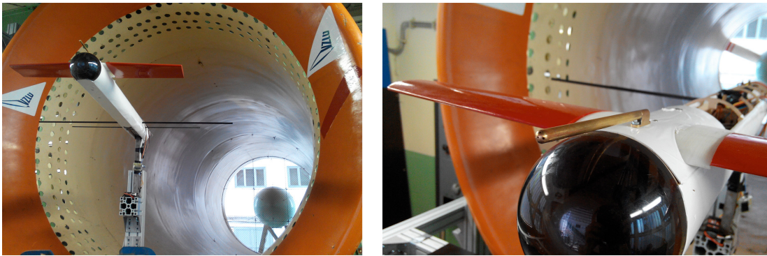
Figure 7.1. Wind tunnel. a) Overall view of wind tunnel with VZLU/CVUT aircraft, b) Detail of the multi-hole pitots tube
